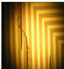
Fig. 3. Separation of metal strips from a silicon substrate
